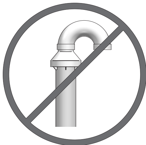
Figure 5-5 Do Not Install U-Bend to Rain Cap
