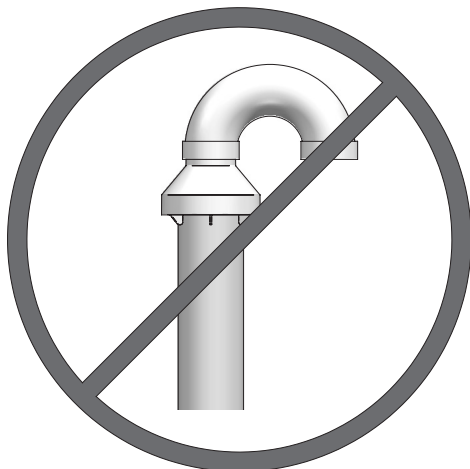
Figure 5-5 Do Not Install U-Bend to Rain Cap
