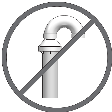
Figure 5-5 Do Not Install U-Bend to Rain Cap
