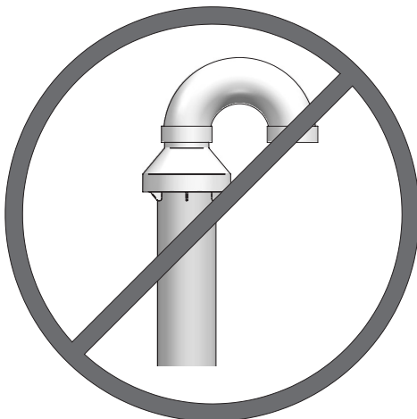
Figure 5-5 Do Not Install U-Bend to Rain Cap
