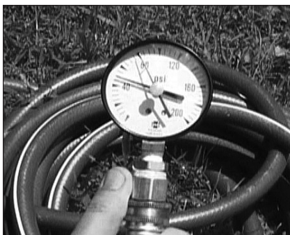
Figure 12. Use a Water Pressure Gauge to make sure your home's water pressure is not too high.
