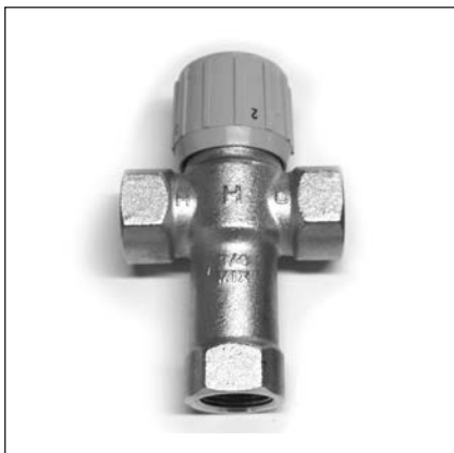
Figure 15. Thermostatic Mixing Valves installed at each point-of-use can help avoid scalding.
