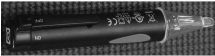
Figure 8. Use a non-contact circuit tester to insure that the power is off before you work on a circuit.
