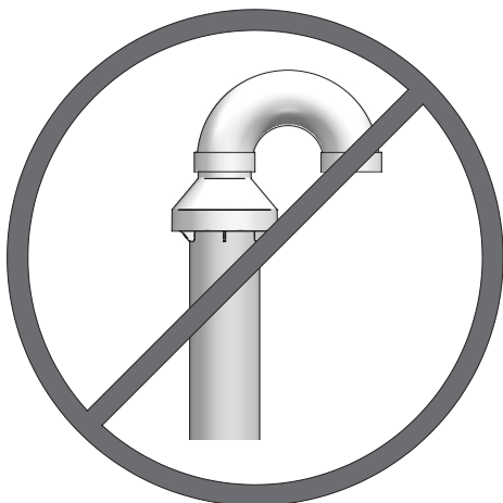
Figure 5-5 Do Not Install U-Bend to Rain Cap
