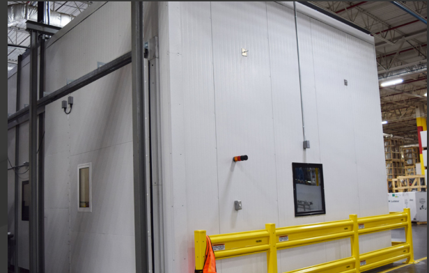
Environmental chamber can be adjusted from -5°F to 140°F
