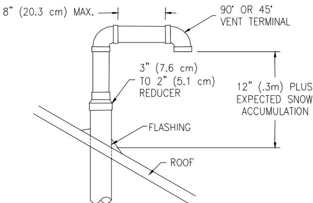
**NOTE:** For installations requiring both horizontal and vertical runs, the following rule must be followed: Total length of straight pipe (both horizontally and vertically) must not exceed the allowable length listed in the Table 7 and 8 for total number of elbows used.
