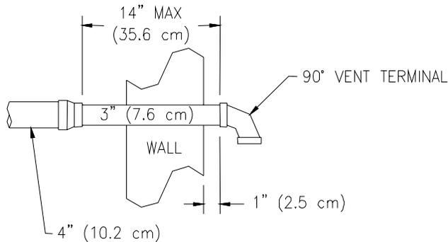
**NOTE: For installations requiring both horizontal and vertical runs, the following rule must be followed: Total length of straight pipe (both horizontally and vertically) must not exceed the allowable length listed in the "Through The Wall" section of the table for total number of elbows used.**
