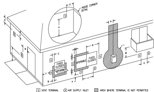
**Figure 1 - Vent Terminal Clearances**
