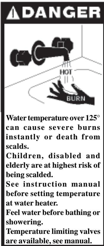
Water temperature over 125° can cause severe burns instantly or death from scalds.
