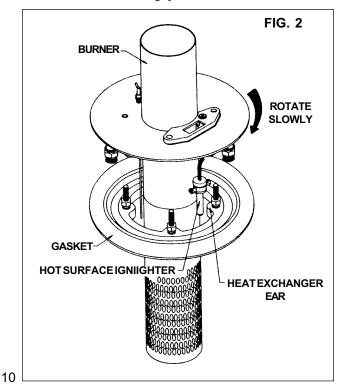
After removing the burner, use a stiff bristle brush to clean the burner ports inside and out. Be sure to remove any foreign material that is in the burner. A water hose can be used to flush contaminants from the burner port area. Dry burner before firing unit. Check for any cracks, holes or deterioration. The burner MUST be replaced when there are holes in both the innner and outer perf material.
