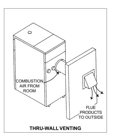
**WARNING:** No substitutions of flue pipe or vent cap material are allowed. Such substitutions would jeopardize the safety and health of inhabitants.
