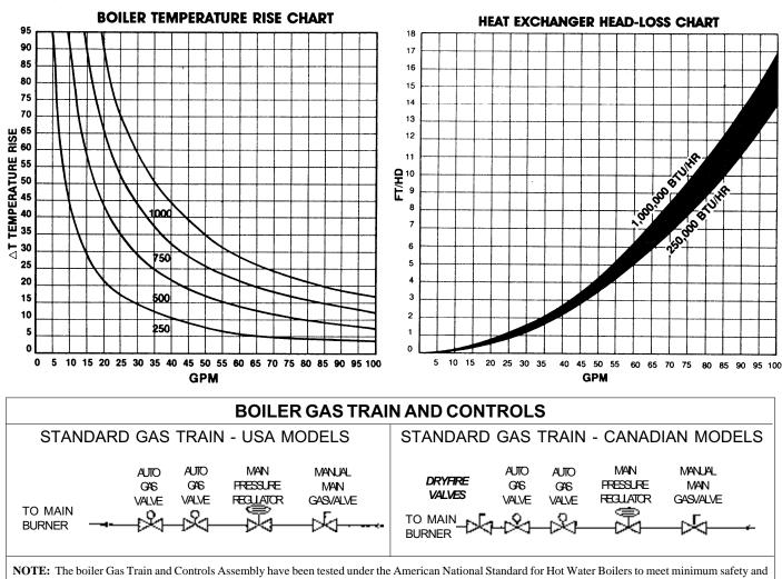
performance criteria such as safe lighting, combustion and safety shutdown operation.
