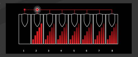
With lead-lag operation, one lead boiler modulates to capacity on demand. As load increases, the system then cascades to additional lag boilers in sequence. The first-on role shifts daily, distributing equal runtimes to each unit.
