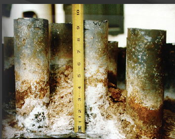
Traditional tank-type water heater flue tubes with nearly 6" of lime scale buildup
