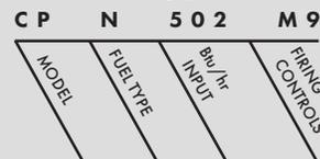
This heater is 500,000 Btu/hr natural gas Copper-Fin 2 Pool Heater. It has M9 firing controls.
