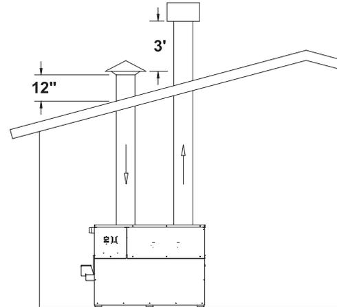
Figure 16 – Roof Top Combustion Air Inlet
