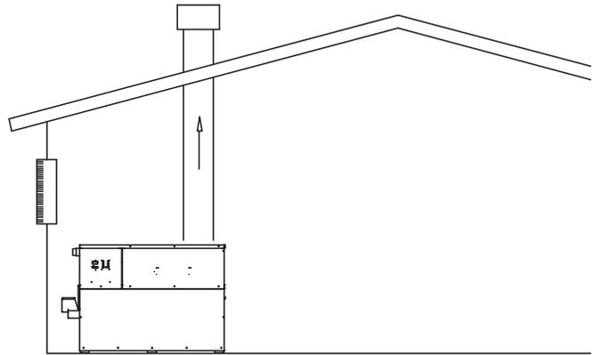
Figure 6 – Outside Combustion Air - Single Opening
