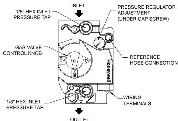
Figure 43 – Combination Gas Valve
