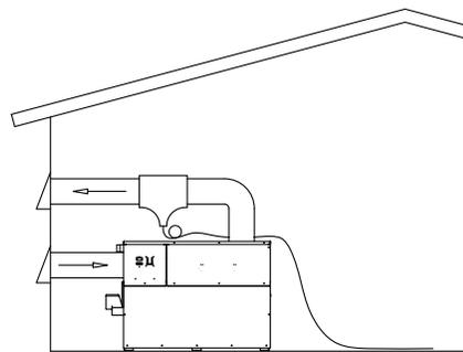
Figure 23B – Aire-Lock Direct Vent (Illustration with Sidewall Vent and Sidewall Combustion Air)
