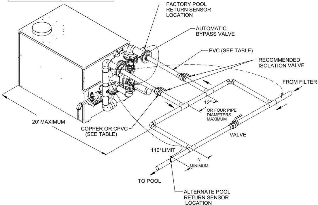
Figure 35 - Heater is Beyond 15 Feet of Pool Piping
