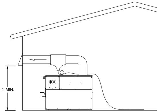
Figure 22 – Sidewall Venting
