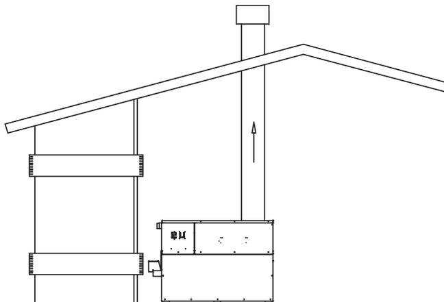
Figure 9 – Combustion Air from Interior Space
