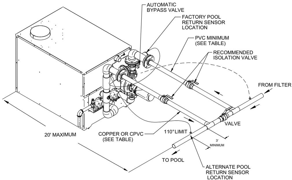
Figure 34 - Heater is Within 15 Feet of Pool Piping
