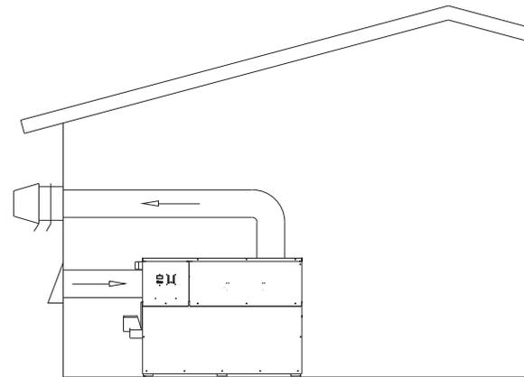
**Figure 23A – Horizontal DirectAire Installation (Illustration with Sidewall Venter and Sidewall Combustion Air)**
