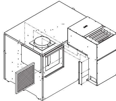
Figure 27 – Outdoor Vent Cap Installed on Rear of Pool Heater
