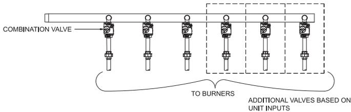
Figure 29 – Typical Pool Heater Gas Train Drawing
