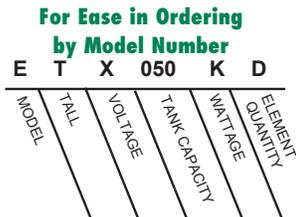
This is a Tall Commercial Electric 480 volt model with a tank capacity of 50 gallons. The upper and lower elements are 4500 watts.
