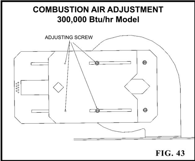
**300,000 Btu/hr Models** - Loosen the four (4) screws holding the air shutter in place. With the fan running, slowly close the air shutter until the low air light comes on. Slowly open the air shutter until the low air light goes off, plus an extra 1/8". Retighten the four (4) holding screws.
