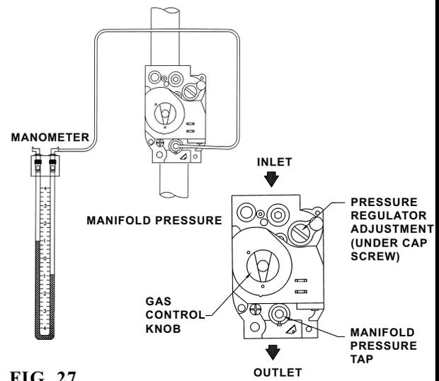
4. Remove the "hex plug, located on manifold piping to burners (300,000 Btu/hr models) or on the "outlet" side of the gas valve (990,000-2,070,000 Btu/hr models) and install a fitting suitable to connect to a manometer or magnahelic gauge. See Figure 26 and 27. Minimum range of scale should be up to 5A" w.c. for natural gas and 10" w.c. for propane gas.
