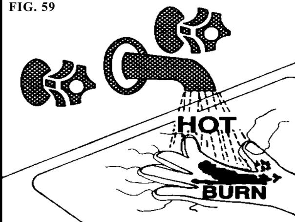
Water temperature over 125°F can cause severe burns instantly or death from scalds.
