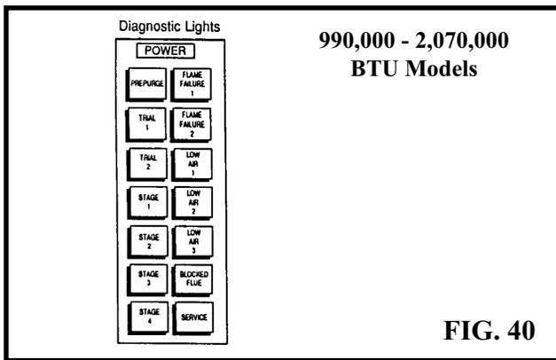
The control panel has an ON/OFF power switch and 15 indicating and diagnostic lights to show all major steps of operation and control sensed malfunctions.
