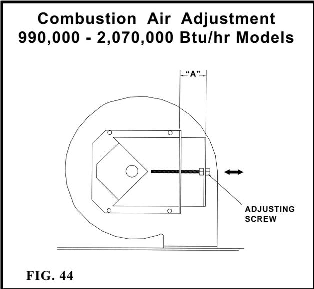
**990,000 through 2,070,000 Btu/hr Models** - The following is a recommended method for setting the differential air pressure ( $\Delta P$ ) for each fan on models with multiple fans.
