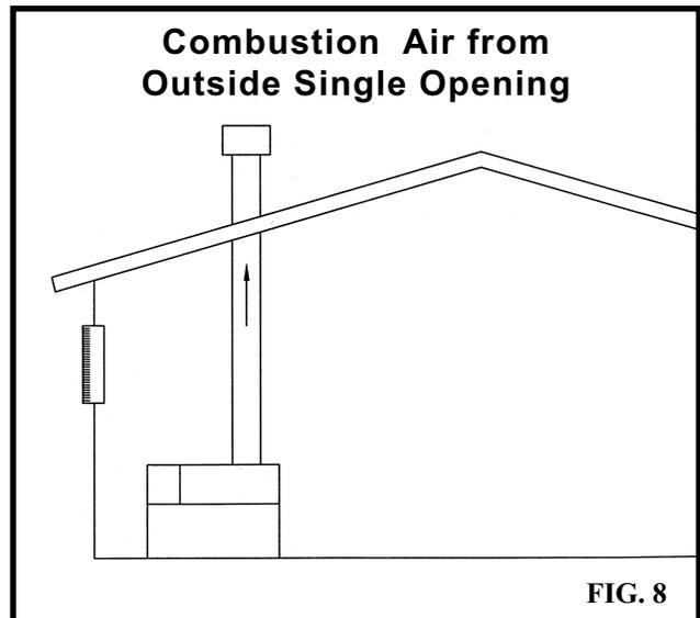
4. If a single combustion air opening is provided to bring combustion air in directly from the outdoors, the opening must be sized based on a minimum free area of one square inch per 3000 Btu ( $7\text{cm}^2$  per kW). This opening must be located within 12" (30cm) of the top of the enclosure.
