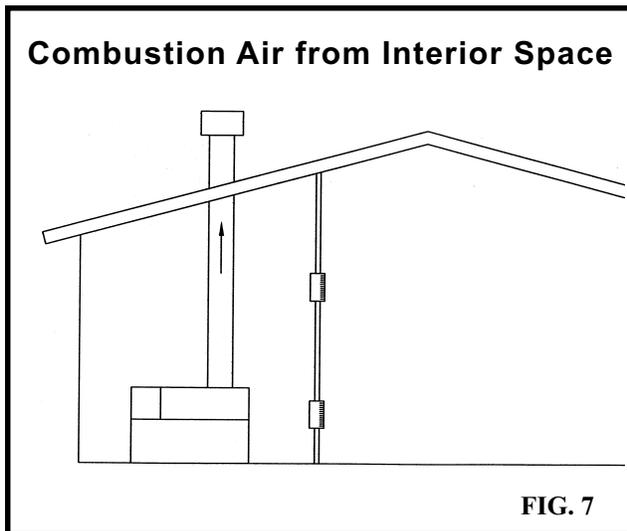
3. If air is taken from another interior space, each of the two openings specified above should have a net free area of one square inch for each 1000 Btu ( $22\text{cm}^2$  per kW) of input, but not less than 100 square inches ( $645\text{cm}^2$ ).
