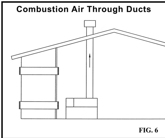
2. If combustion and ventilation air is taken from the outdoors using a duct to deliver to the mechanical room, each of the two openings should be sized based on a minimum free area of one square inch per 2000 Btu ( $11\text{cm}^2$  per kW).
