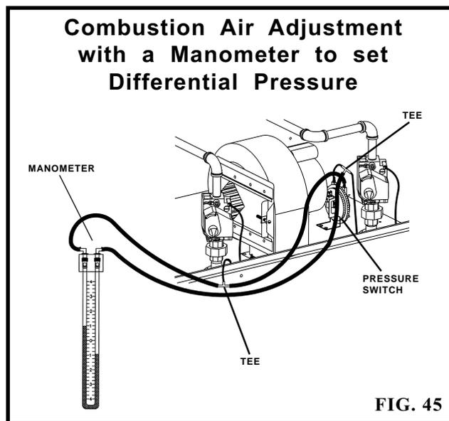
The “⊕” connection on the manometer connects to the tubing from the units front chamber and the “⊖” connection on the manometer connects to the tubing from the burner venturi.
