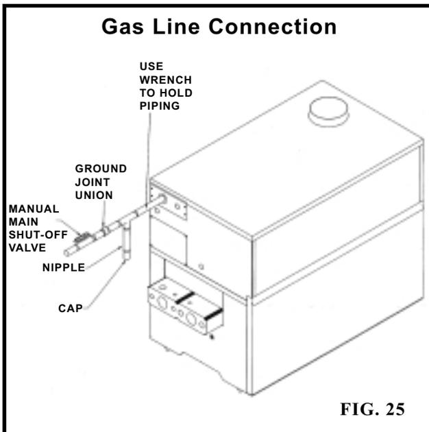
All gas connections must be made with pipe joint compound resistant to the action of liquefied petroleum and natural gasses. All piping must comply with local codes and ordinances. Tubing installations must comply with approved standards and practices.
