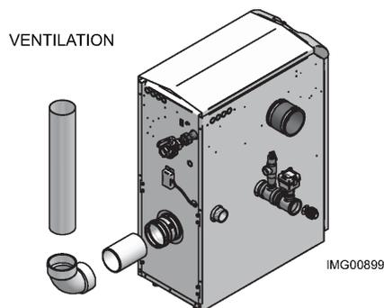
LE TUYAU de 3 ou 4" EN CPVC FOURNI AVEC LE CHAUFFE-EAU DOIT ÊTRE UTILISÉ POUR LE RACCORDEMENT DE LA VENTILATION
