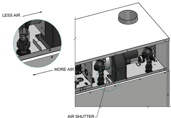
**Figure 2-3** Adjusting air shutter - 990,000 - 2,070,000 Btu/hr Models
