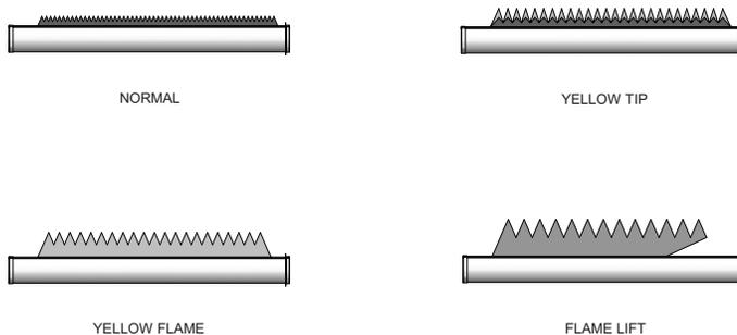
**Normal Flame:** A normal flame at 100% of burner input is blue, with slight yellow tips, a well defined flame and no flame lifting.
