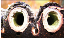
Scale buildup from untreated water.
