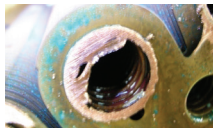
Picture shows a clean HX with treatment.
