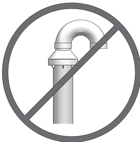
Figure 4-5 Do Not Install U-Bent to Rain Cap
