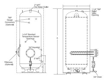
♦ The manway is optional on 257 and 318 gallon glass-lined tanks. The manway is standard on 432 gallon glass lined tanks and larger. The manway is standard on all cement lined tanks.
