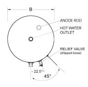
The "Hot Water Outlet" connection is Female NPT. All other connections are Male NPT.
