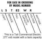
This is a Tall Commercial Electric 277 volt model with a tank capacity of 80 gallons. The upper and lower elements are 6100 watts.
