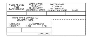
The volts, phase, and watts information of the rating plate must be modified by covering them with conversion label provided in the conversion kit. Be sure the new ratings on the label match the conversion you have just completed.
