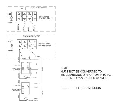
Figure 1. Four-Wire Circuit for Dual-Element Heater
