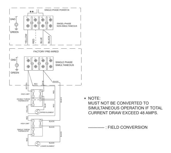
Figure 1. Four-Wire Circuit for Dual-Element Heater
