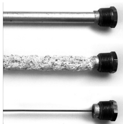
Figure 14 - Anode rods from new to (top) to partially depleted (middle) to fully depleted stages (bottom).
