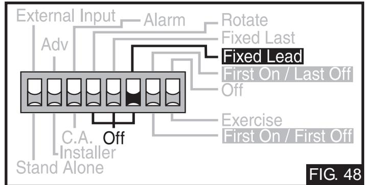
The First On / Last Off or First On / First Off DIP switch selects whether the first boiler is the first to stage on and the last to stage off or the first to stage on and the first to stage off. This DIP switch is only active when the Rotate / Off DIP switch is set to Rotate and the Fixed Lead / Off DIP switch is set to Fixed Lead (FIG. 49).
