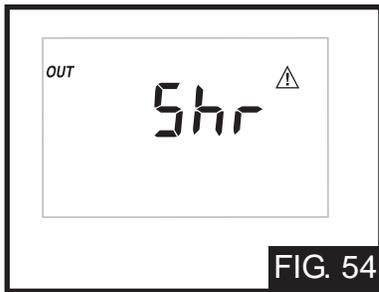
The control is no longer able to read the outdoor sensor due to a short circuit (FIG. 54). In this case the control assumes an outdoor temperature of 32°F (0°C) and continues operation. Locate and repair the problem as described in INS7141. To clear the error message from the control after the sensor has been repaired, press either the Menu or Item button. This error message only occurs if the External Input / Stand Alone DIP switch is set to Stand Alone.
