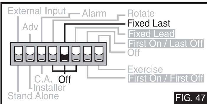
The Fixed Lead / Off DIP switch selects whether or not the first boiler is to be included in the rotation sequence. If the DIP switch is set to Fixed Lead, the first boiler is always the first to fire (FIG. 48). This DIP switch is only active when the Rotate / Off DIP switch is set to Rotate.
