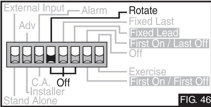
The Fixed Last / Off DIP switch selects whether or not the last boiler is to be included in the rotation sequence. If the DIP switch is set to Fixed Last, the last boiler is always the last to fire (FIG. 47). This DIP switch is only active when the Rotate / Off DIP switch is set to Rotate.
