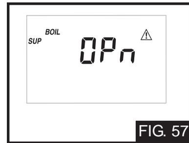
The control is no longer able to read the boiler supply sensor due to an open circuit (FIG. 57). The control will not operate the boiler(s) until the sensor is repaired. Locate and repair the problem as described in INS7141. To clear the error message from the control after the sensor has been repaired, press either the Menu or Item button.
