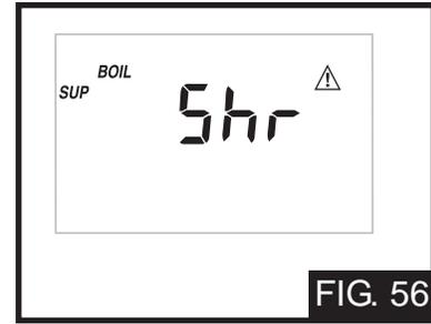
The control is no longer able to read the boiler supply sensor due to a short circuit (FIG. 56). The control will not operate the boiler(s) until the sensor is repaired. Locate and repair the problem as described in INS7141. To clear the error message from the control after the sensor has been repaired, press either the Menu or Item button.
