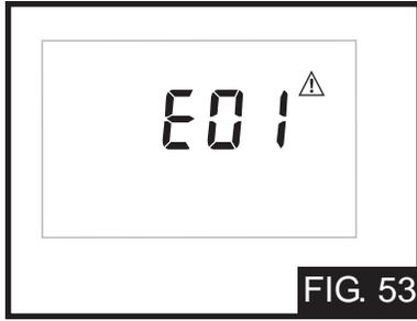
The control was unable to read a piece of information stored in its memory (FIG. 53). Because of this, the control was required to reload the factory settings into all of the items in the ADJUST menu. The control will stop operation until all of the items in the ADJUST menu of the control have been checked by the user or installer.
