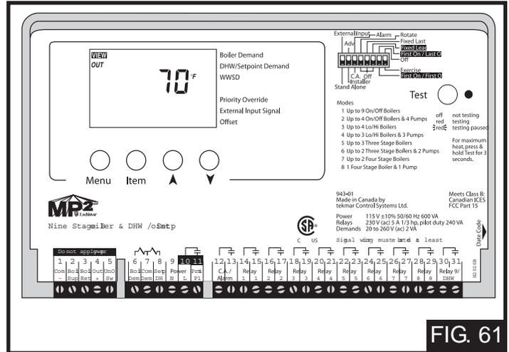
The control has detected no increase in the supply water temperature within the BOIL Alarm time setting. Check to see if the boilers are operating properly using the Test button. To reset the alarm, press and hold the up and down arrow buttons for 5 seconds while in the VIEW menu.
