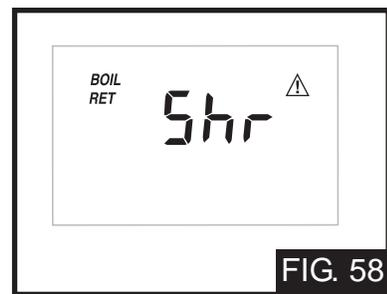
The control is no longer able to read the boiler return sensor due to a short circuit (FIG. 58). The control will continue to operate normally. Locate and repair the problem as described in INS7141. To clear the error message from the control after the sensor has been repaired, press either the Menu or Item button.
