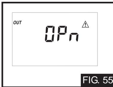
The control is no longer able to read the outdoor sensor due to an open circuit (FIG. 55). In this case the control assumes an outdoor temperature of 32°F (0°C) and continues operation. Locate and repair the problem as described in INS7141. To clear the error message from the control after the sensor has been repaired, press either the Menu or Item button. This error message only occurs if the External Input / Stand Alone DIP switch is set to Stand Alone.
