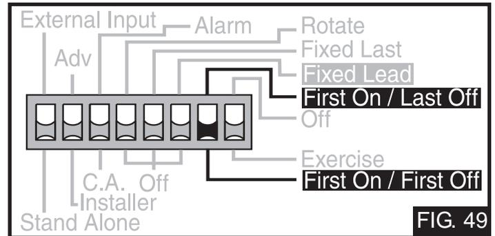
The Off / Exercise DIP switch selects whether or not the control is to exercise the primary pump and boiler pumps (FIG. 50). If the DIP switch is set to Exercise, the pumps are operated for 10 seconds after every three days of inactivity.
