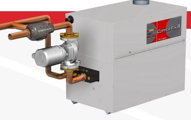
The Lochinvar LTV Low Temperature Valve is shipped separately and can be easily incorporated into the field-installed primary/secondary boiler piping. (2" LTV Valve shown installed on CHN752)
